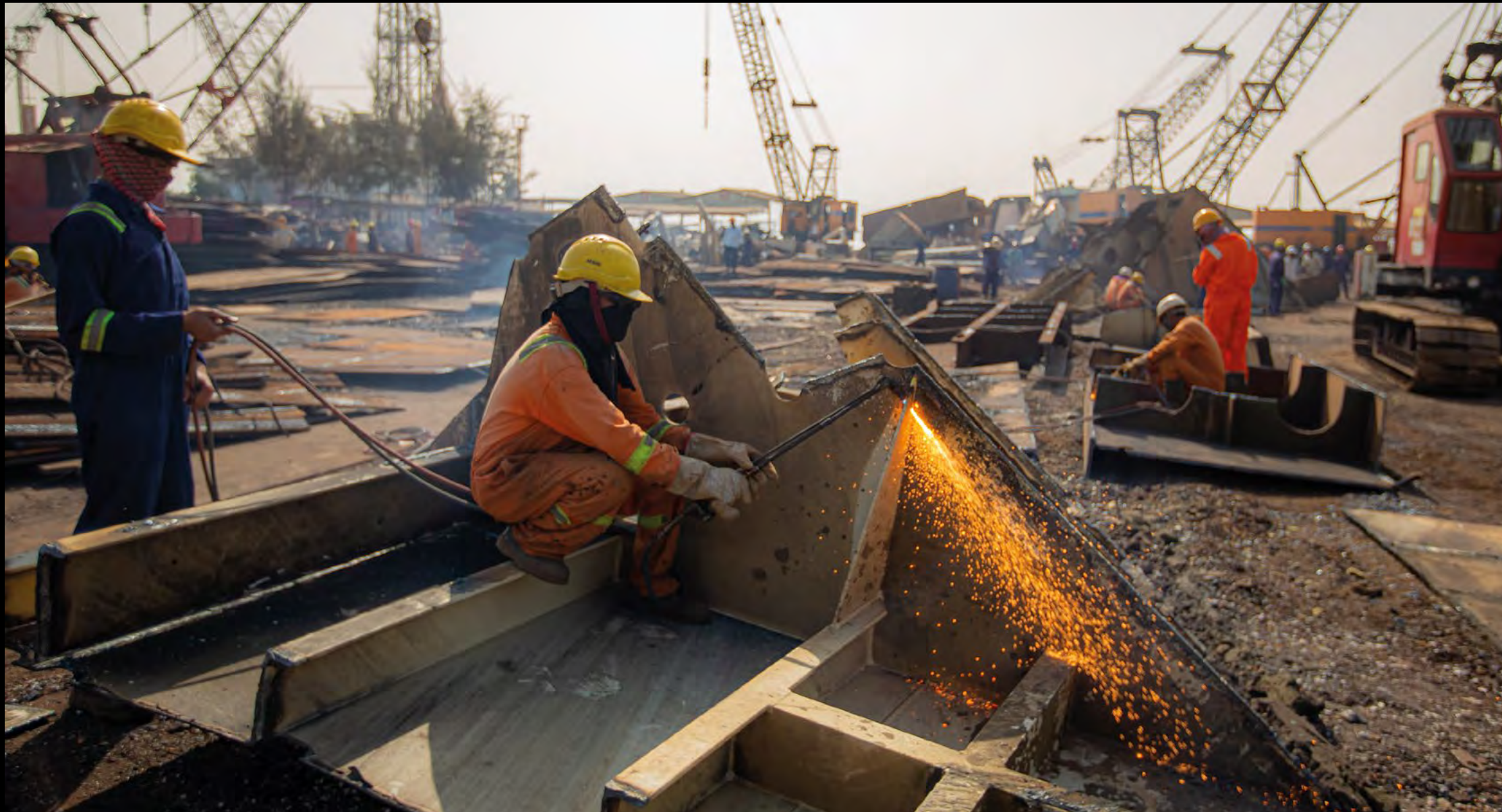
ABOVE: Cutting torches are used to cut the steel plates from the ship into smaller pieces. These are finally melted down into usable bars.
